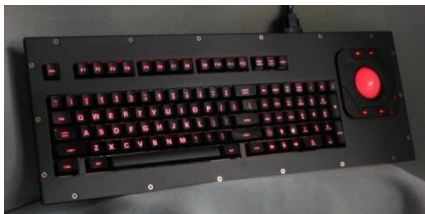
Backlit Panel mount with 2" DuraTrackball
